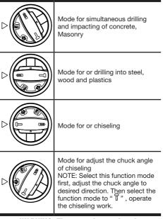
WARNING: The operating mode selector switch may be actuated only at a standstill.
